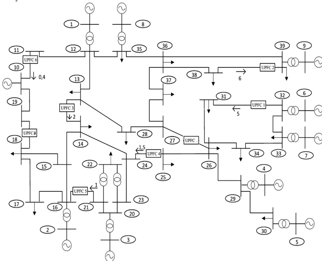
Fig. 7. Modified New England network with 8 UPFC
