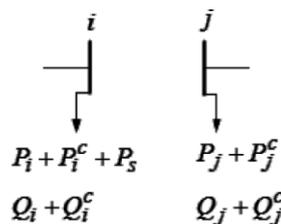
Fig. 5. Injected powers in the bus bars with the inclusion of UPFC
