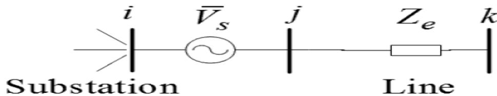
Fig. 2. Equivalent model of UPFC in the electric network
