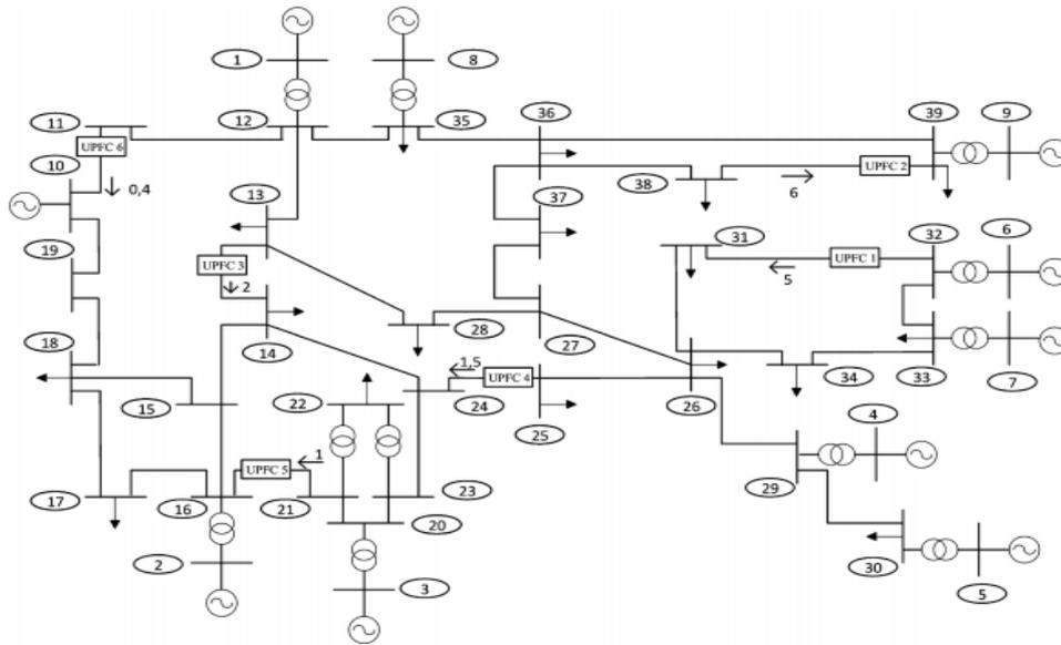
**Fig. 6.** Modified New England network with 6 UPFC
